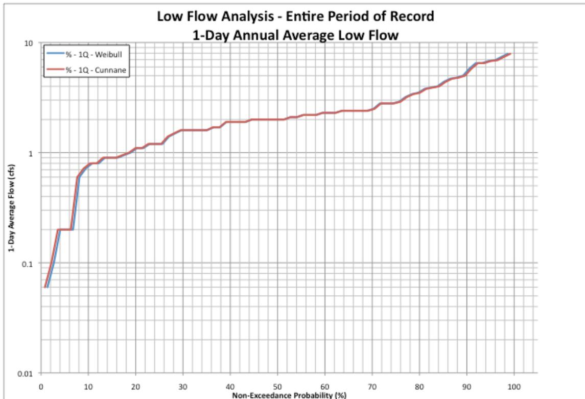
**Figure 1.12:** Low flow frequency analysis for USGS gauge #11418500 on Deer Creek,  $d=1$ , using the Weibull (blue) and Cunnane (red) plotting methods.
