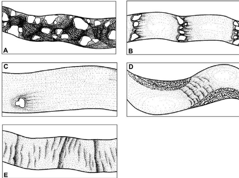
**Figure 2.2:** Schematic Plan Form of Mountain Stream Channel Classifications: **A)** Cascade; **B)** Step Pool; **C)** Plane Bed; **D)** Pool Riffle; **E)** Dune Riffle (Reprinted from Montgomery and Buffington 1997).
