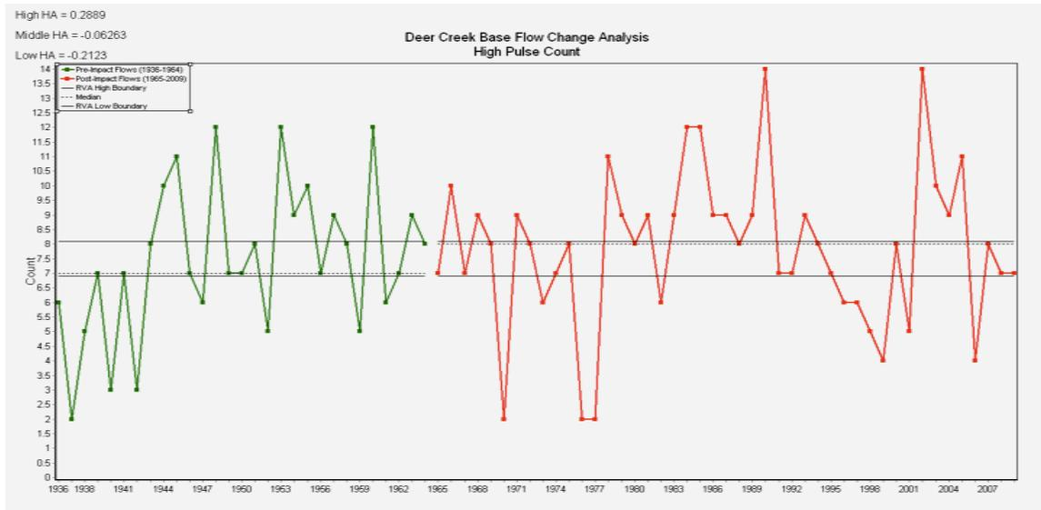
**Figure 1.23:** IHA software high flow pulse analysis, high pulse count (frequency) plot.
