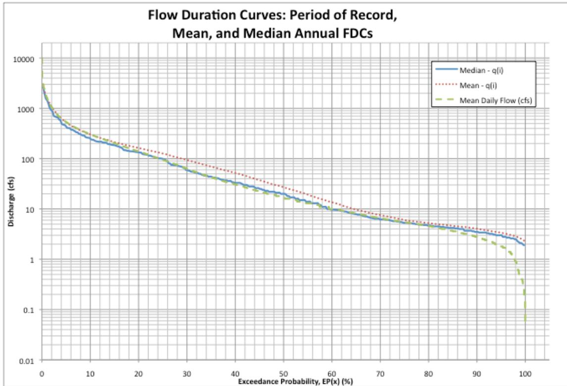
**Figure 1.14:** Flow Duration Curves: Period-of-record (green-Mean Daily Flow (cfs)), median-annual (blue-Median –  $q(i)$ ), and mean-annual (red-Mean –  $q(i)$ ).
