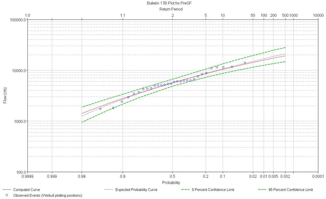
**Figure 1.15:** Results of the PreSF period (1935-1964) flood frequency analysis, n=30.
