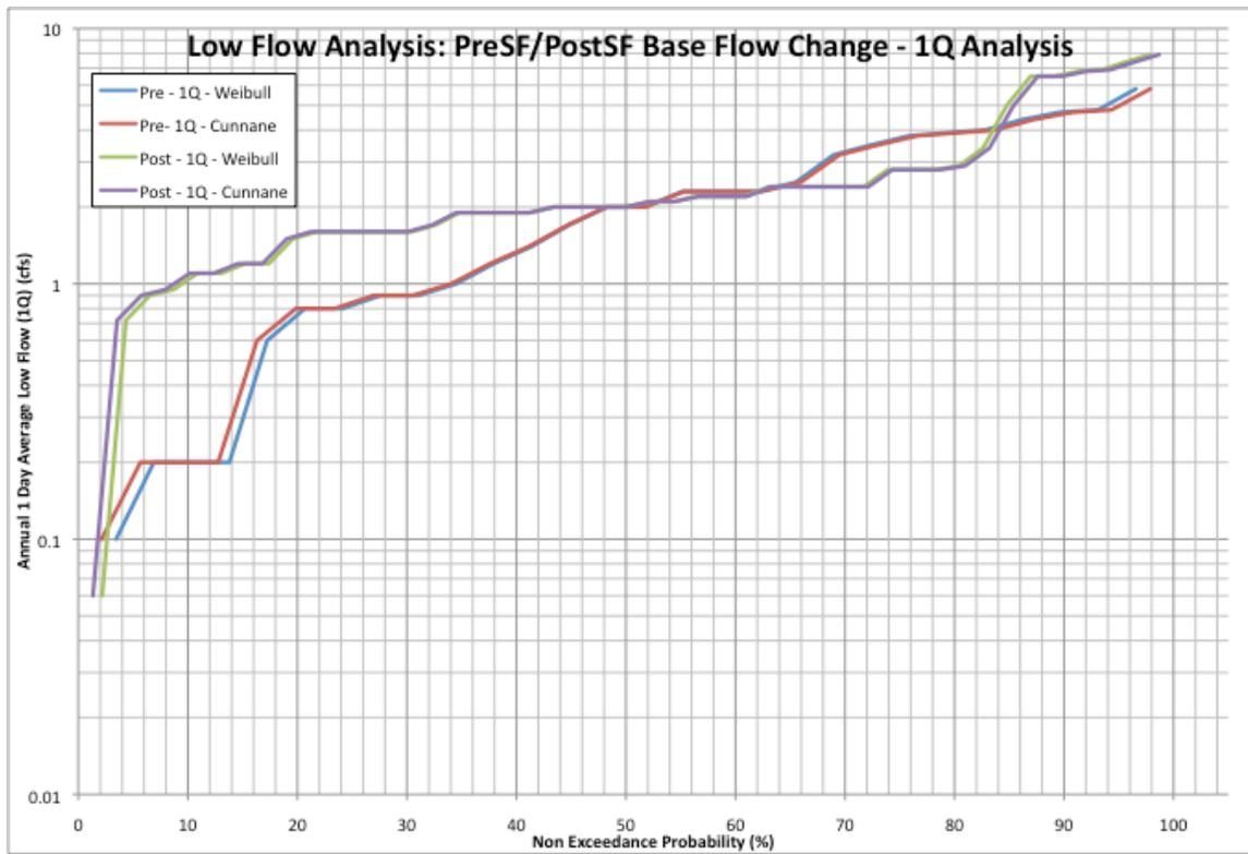
**Figure 1.17:** Results of the two-period low flow frequency analysis,  $d=1$ , annual 1-day average low flow.
