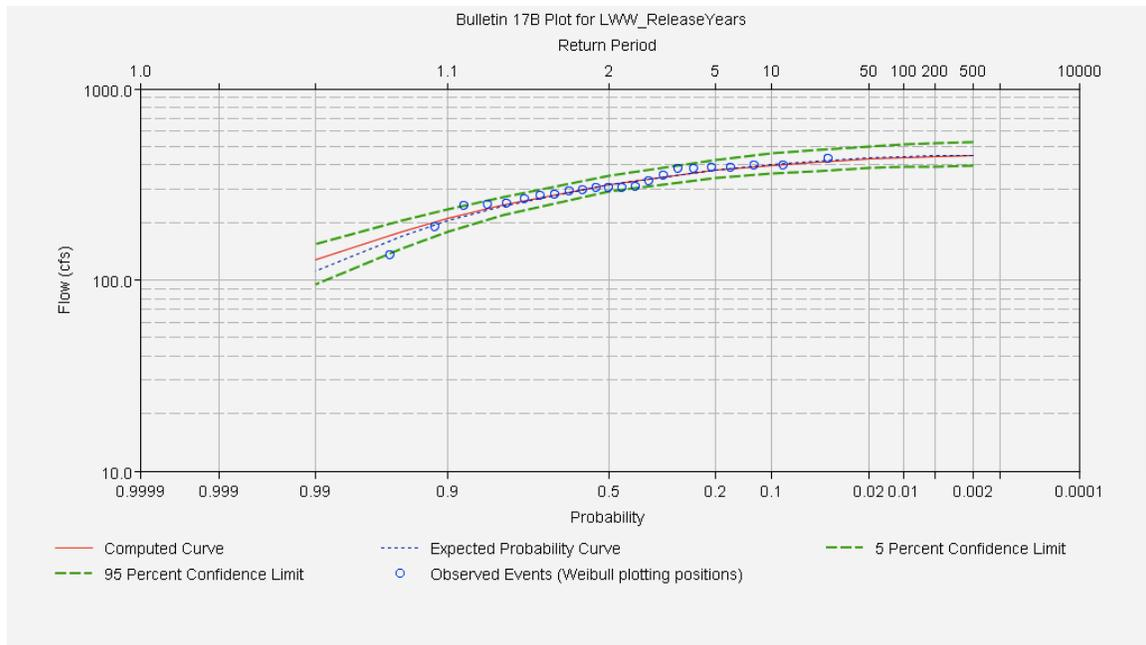
**Figure 1.38:** Results of the HEC-SSP flood frequency analysis for years in which drawdown releases occurred (n=23).
