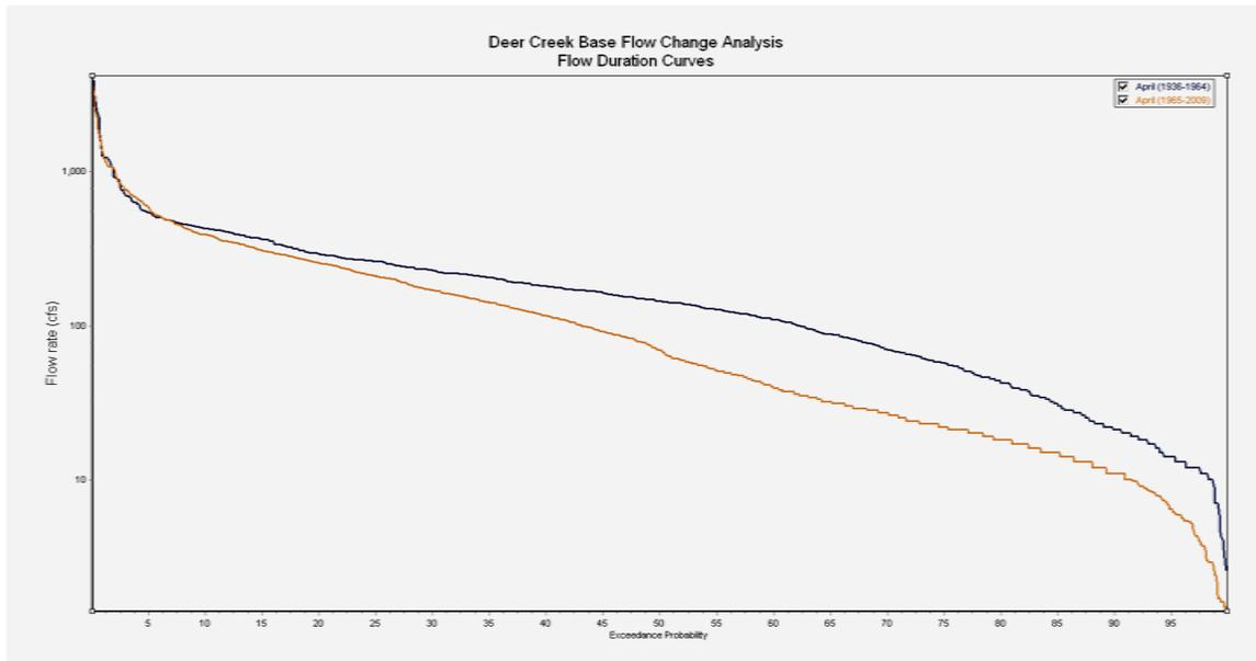
**Figure 1.32:** IHA software monthly flow duration curves for the month of April, with the PreSF period plotted dark blue and the PostSF period orange.
