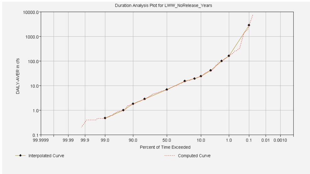
**Figure 1.39:** Graph showing the results of the duration analysis for years in which no drawdown release occurred (n=52).
