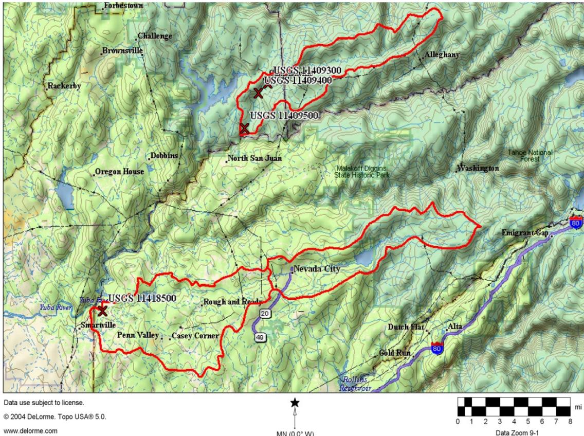
**Figure 1.5:** Locations of USGS stream flow gauges (marked with red Xs) on Deer Creek and Oregon Creek. There are three gauges on Oregon Creek and one on Deer Creek.
