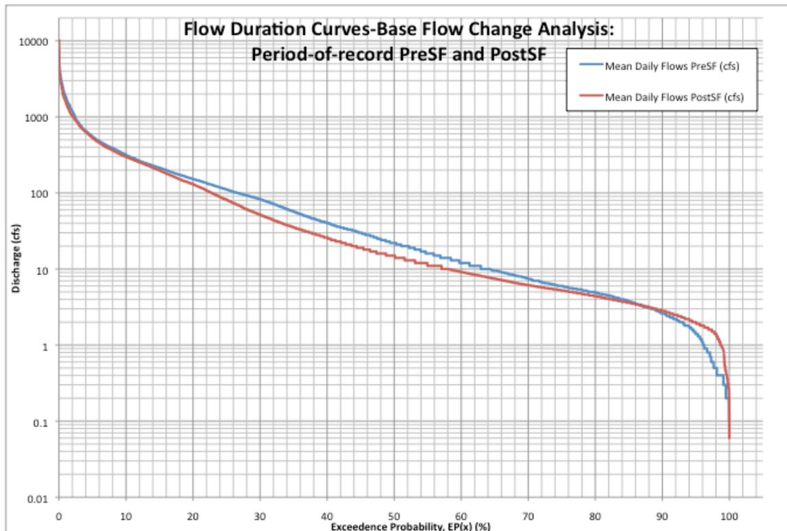
Figure 1.21: Flow duration curves to compare the period before (PreSF) and after (PostSF) water year 1965, using the period-of-record method and plotting mean daily flows.
