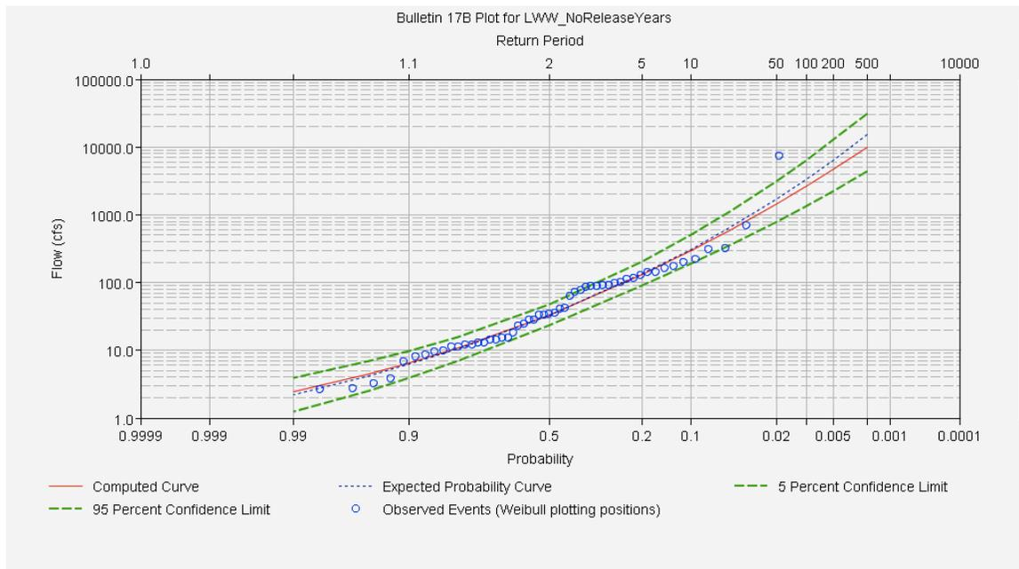
**Figure 1.37:** Results of the HEC-SSP flood frequency analysis for years in which no drawdown release occurred ( $n=52$ ).
