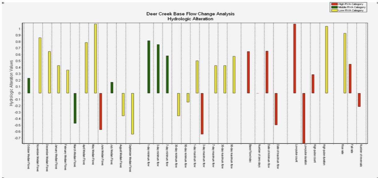
**Figure 1.35:** Graph showing results of the IHA analysis, displaying the areas of greatest hydrologic alteration for each IHA parameter analyzed.
