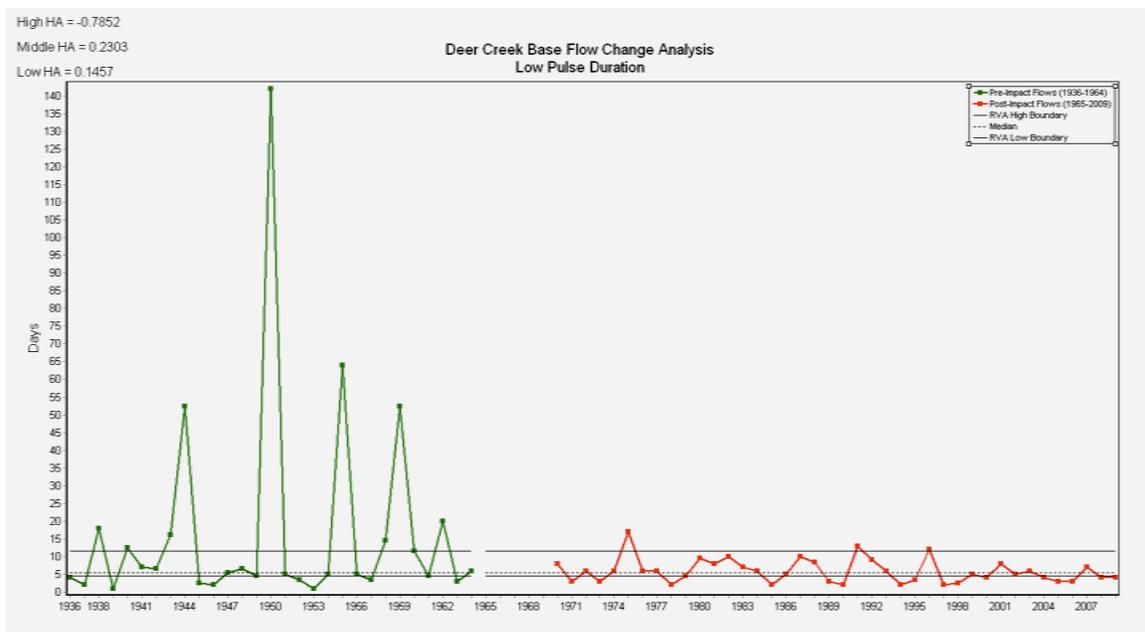
**Figure 1.28:** IHA software low flow pulse analysis, low pulse duration plot.
