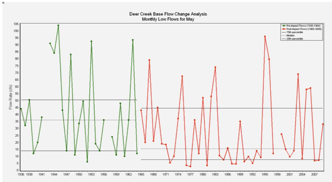
**Figure 1.30:** Summary plot of the IHA software EFC monthly low flows analysis, using the non-parametric method, and plotting alterations to low flows in the month of May.
