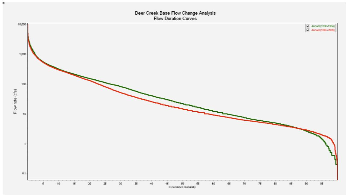
**Figure 1.31:** IHA software Annual Flow Duration Curves for PreSF and PostSF, with the PreSF period plotted green and the PostSF period red.
