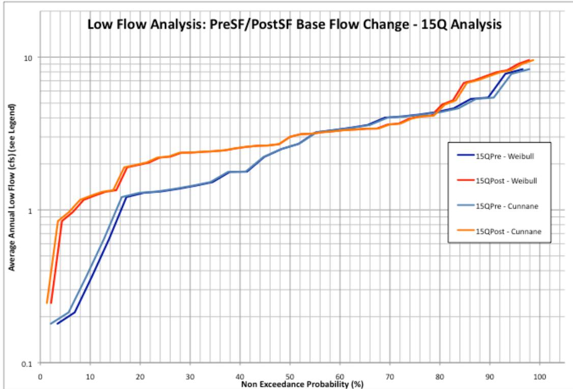
Figure 1.18: Results of the two period low flow frequency analysis, d=15, annual 15-day average low flow.
