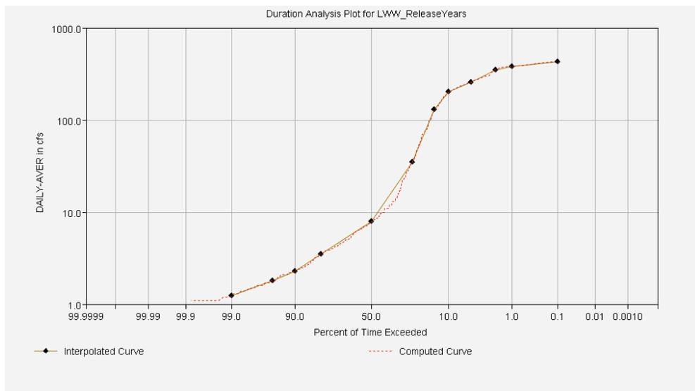
**Figure 1.40:** Graph showing the results of the duration analysis for years in which drawdown releases occurred (n=23).
