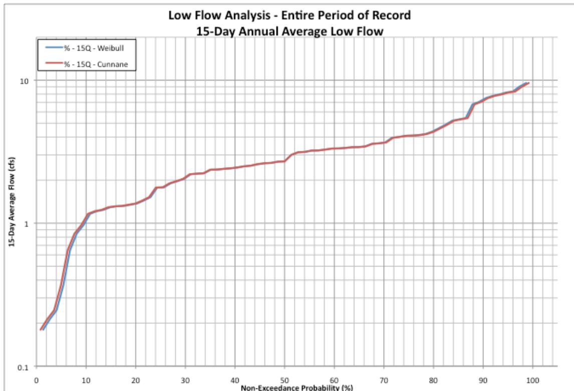
**Figure 1.13:** Low flow frequency analysis for USGS gauge #11418500 on Deer Creek,  $d=15$ , using the Weibull (blue) and Cunnane (red) plotting methods.
