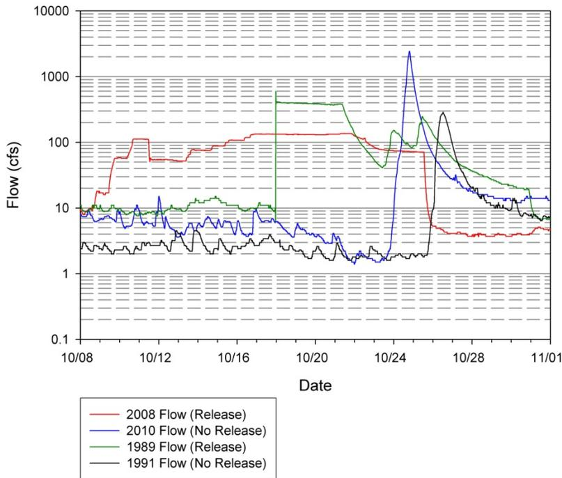
**Figure 1.44:** Comparison of natural streamflow hydrographs against two drawdown releases. Both a drawdown release and natural storm flow are present in the 1989 graph.
