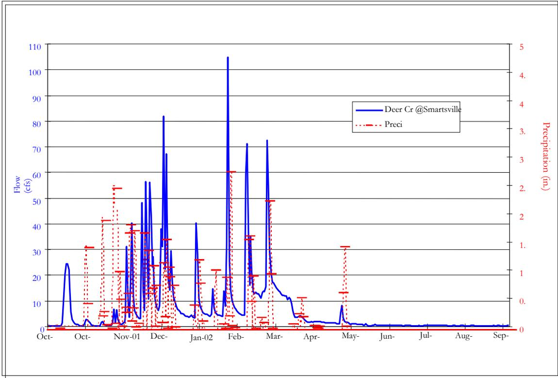
**Figure 1.3:** Water Year 2002 precipitation at Nevada City (right axis) and Deer Creek stream flow at Smartsville (left axis; USGS #11418500, daily mean discharge).
