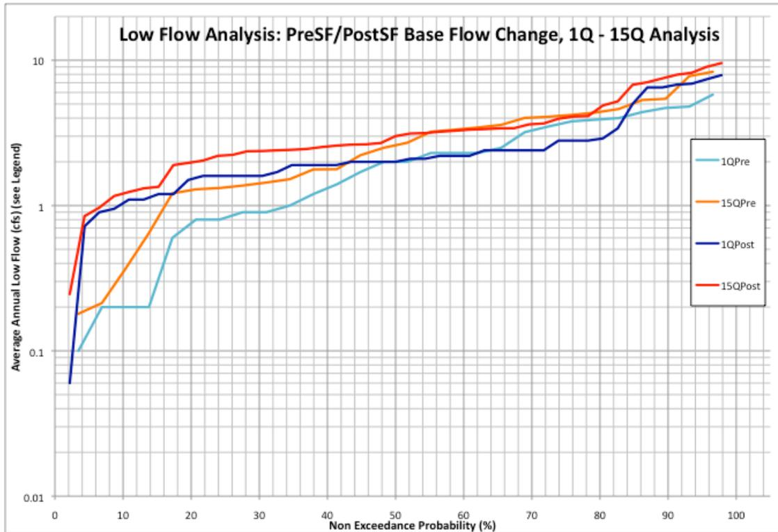
**Figure 1.19:** Results of the two-period low flow frequency analysis,  $d=1$  and  $d=15$ , using the Weibull plotting method.
